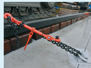
Crane Stop and Securing gear
